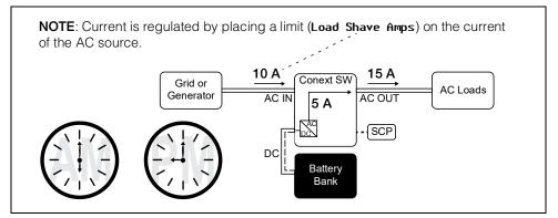
Figure 1-2 Load Shaving in Action
