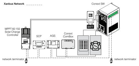
Figure 2-1 Xanbus System Components
