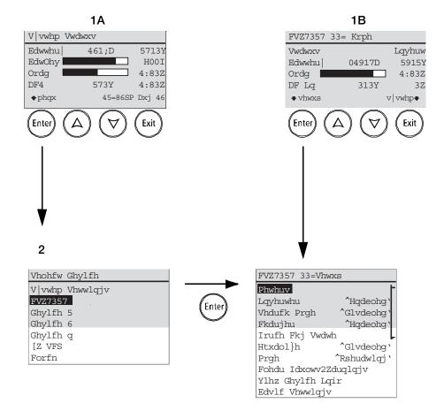
Figure 3-7 Navigate To Conext SW Setup Menu
