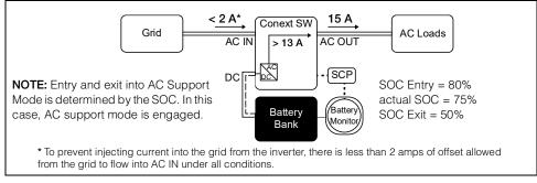
Figure 1-3 AC Support Mode using SOC
