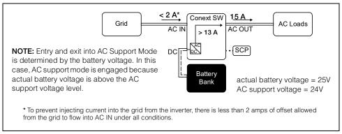
Figure 1-6 Regular AC Support without Xanbus Devices
