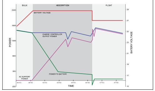
Figure 1-5 Enhanced AC Support Charge Cycle
