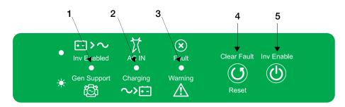
Figure 2-3 Front Panel Buttons and Status LEDs
