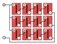
FIGURE 5: Three Parallel Strings. Series/Parallel
