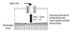
FIGURE 7: Electrolyte level
