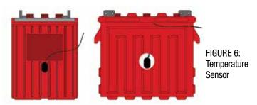
**Dual-Container Models** - Remove case cover. Mount sensor to the side of internal cell below liquid level. Replace the cover and re-seal around terminals with silicone.
