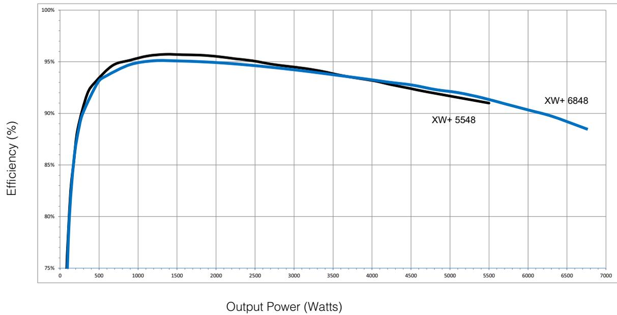
Figure A-3 Inverting Efficiency (Typical)
