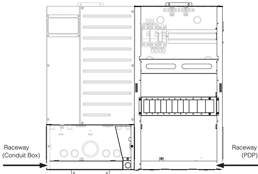
**Figure 2-11** Example of raceways in a single-inverter system
