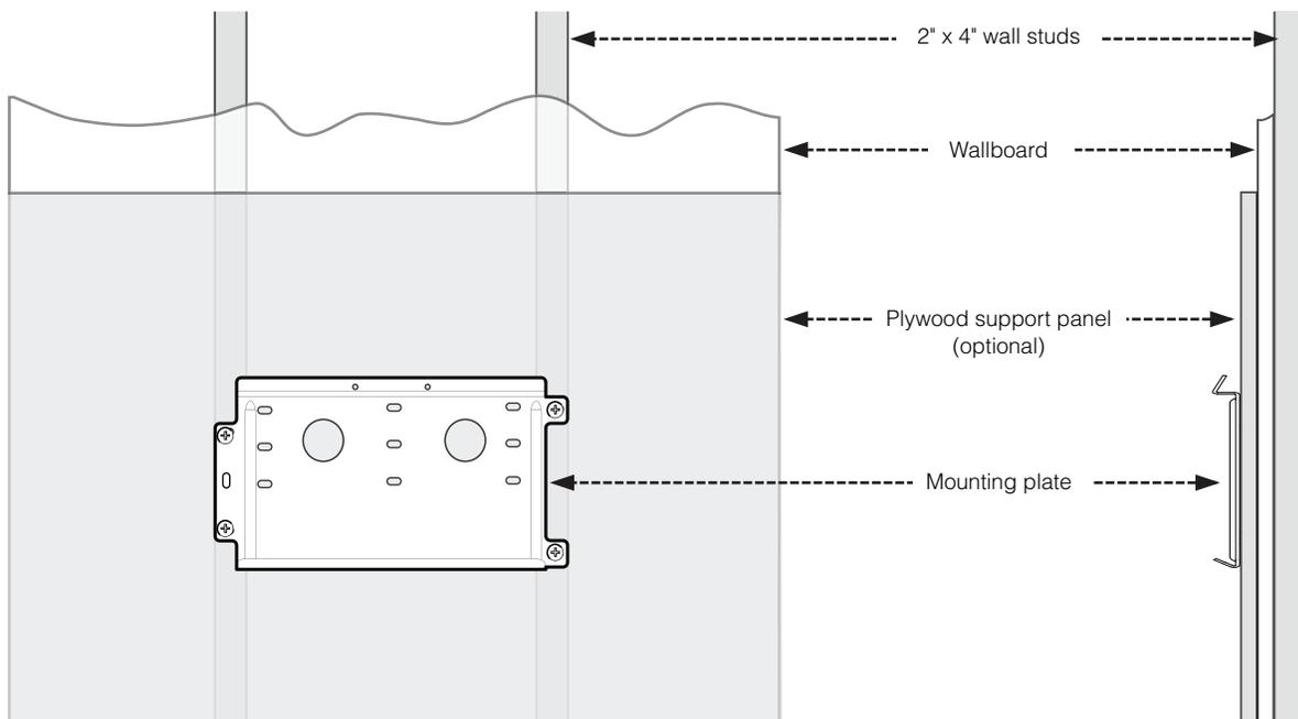
**Figure 2-5** Mounting plate centered on wall studs
