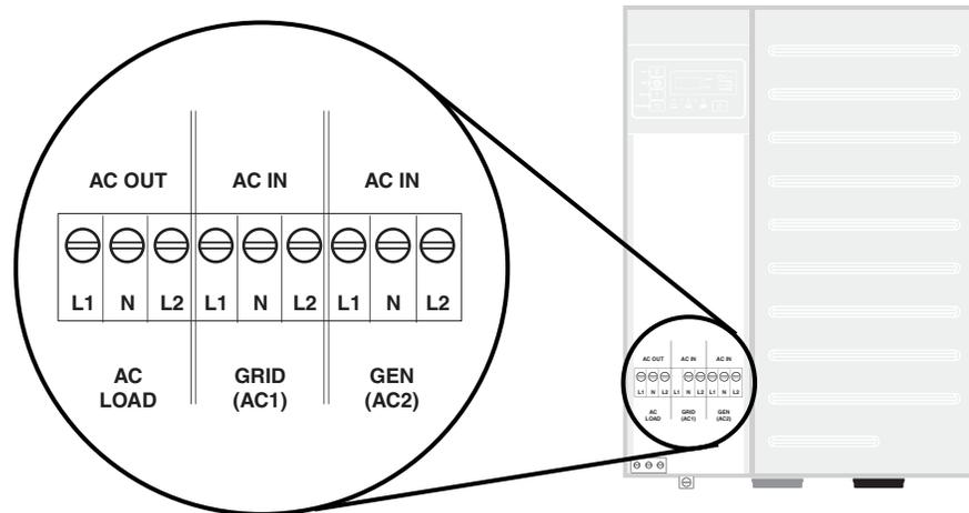
**Figure 3-10** AC terminal block
