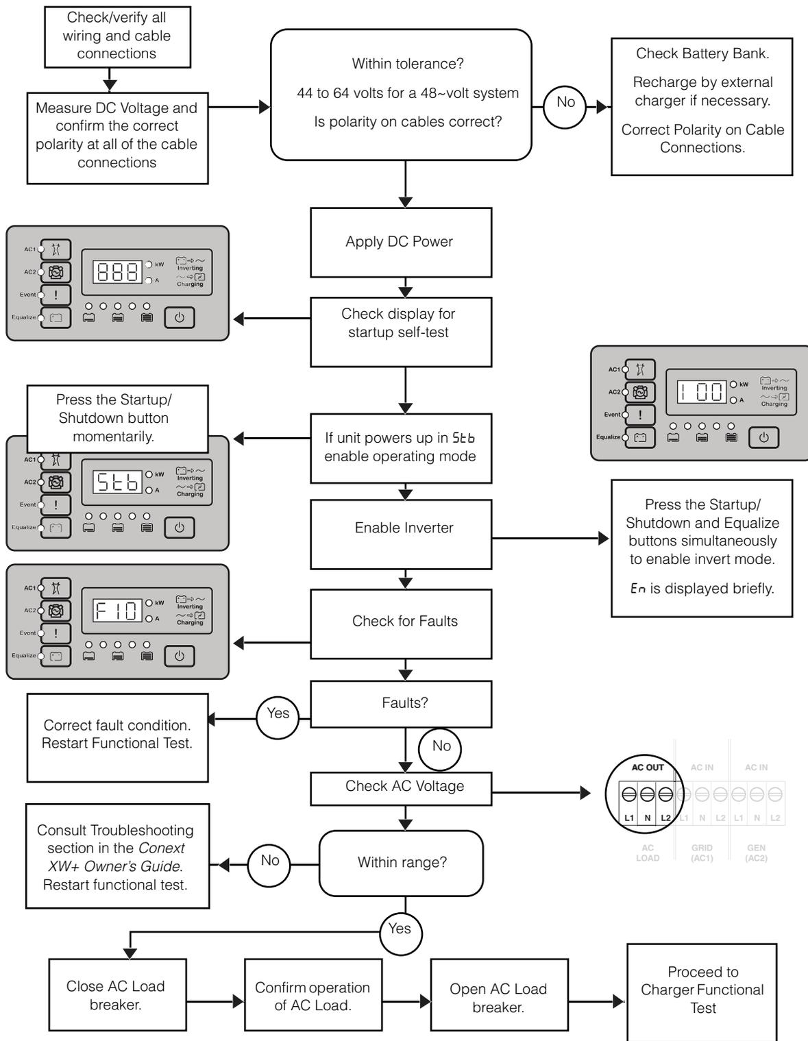
Figure 3-22 Functional Test for Single Inverter Systems
