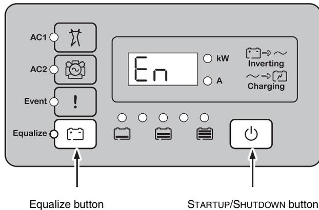
**Figure 3-18** Enabled mode
