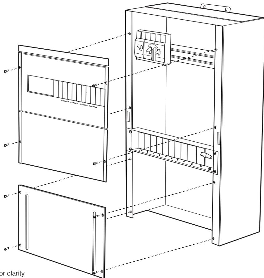
**Figure 3-2** Conext XW+ Power Distribution Panel faceplate removal
