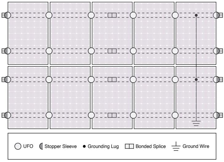
Approved Enphase microinverters can provide equipment grounding of IronRidge systems, eliminating the need for grounding lugs and field installed equipment ground conductors (EGC). A minimum of two microinverters mounted to the same rail and connected to the same Engage cable is required. Refer to installation manuals for additional details.
