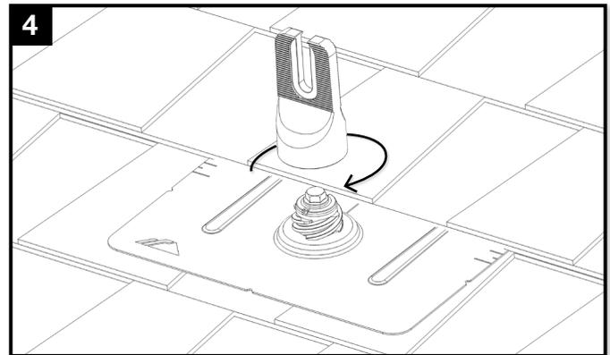
Place Cap onto flashing in desired orientation for E/W or N/S rails and rotate 180 degrees. FlashFoot 2 is now installed and ready for IronRidge XR Rails.
